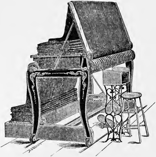
BURLING AND SPECKING MACHINE, FOR REMOVING BURRS, KNOTS AND SPECKS FROM THE FACE OF FABRICS.
